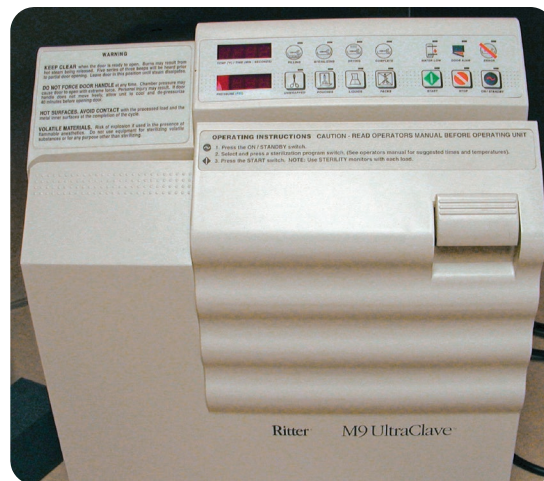
FIGURE 35-6 Steam autoclaving is the most common method of sterilizing instruments and equipment. Understanding the gauges and timer is essential to proper operation of an autoclave.
