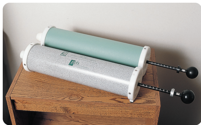
FIGURE 49-23 A calibration syringe delivers a fixed volume of air.
