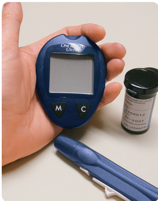
FIGURE 45-3 A handheld glucometer translates the amount of reflected light into the level of glucose in a blood sample.
