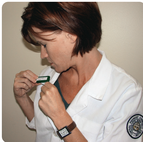
FIGURE 50-9 A radiation exposure badge contains a film that registers the levels of radiation to which a medical staff member is exposed at work.
