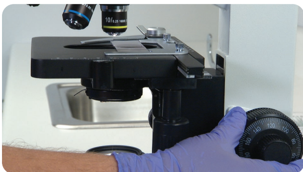
FIGURE Procedure 45-1 Step 9 When lowering the objective toward the stage and specimen slide, observe the microscope from the side to be sure you do not hit the stage with the objective and crack the slide.
