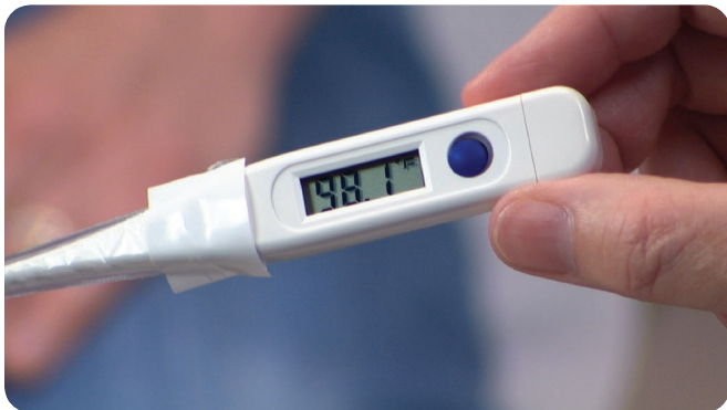
FIGURE 37-1 An electronic digital thermometer provides a digital readout of the patient's temperature.
